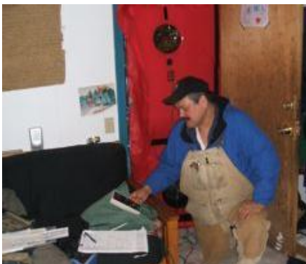
ABSN Field Manager collecting blower-door test figures
